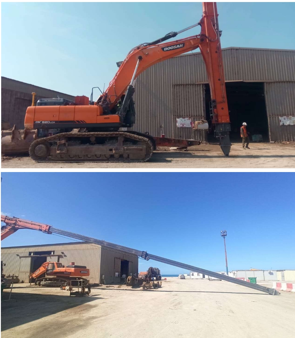
Figure 1 - Telescopic hex; Top: Stick fully retracted; Bottom: Stick fully extended
