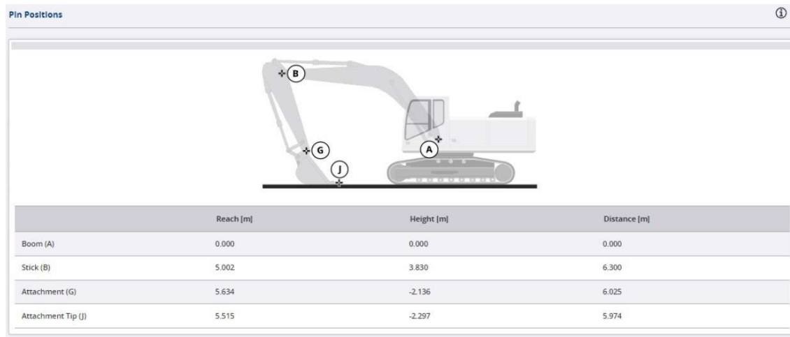
Figure 11 – Machine readings for EW 2D part validation.
